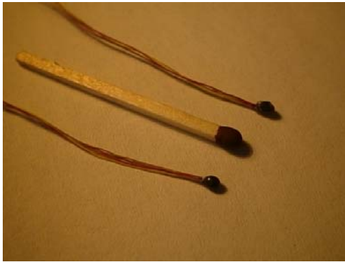
Fig. 2.: The hot ball sensor (left) for measuring thermal conductivity and the corresponding temperature response (right).
