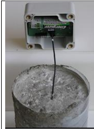
Fig. 4.: Experimental arrangement for measuring setting point by RTM 1.01
